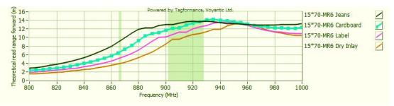
Sensitivity&Read Range Test power: 4W EIRP
